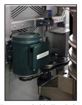
Proven, reliable Tru-Balance drive mechanism provides the gentle, gyratory sifting motion for which our sifters are known.
