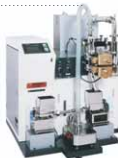
Closed circuit system with jet mill
