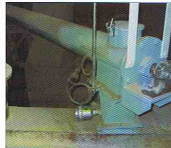
Microwave Flow Switch for screw feeder
