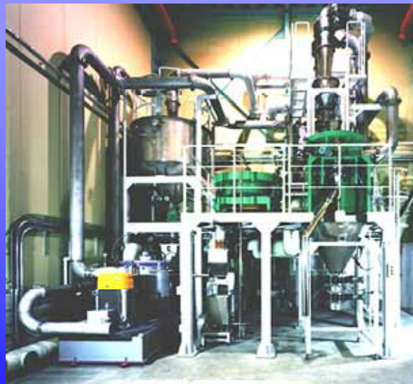
Toner manufacturing plant using the mechanical mill
