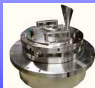
A new classifier for fine classification
