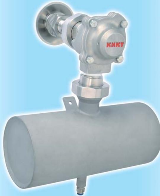
The PUL BLAS® is recommended for eliminating bridges, rat holes or side wall build-up on vessel walls that may occur in various hoppers or tanks. The Air Pulser delivers maximum effect with minimum air quantity.
