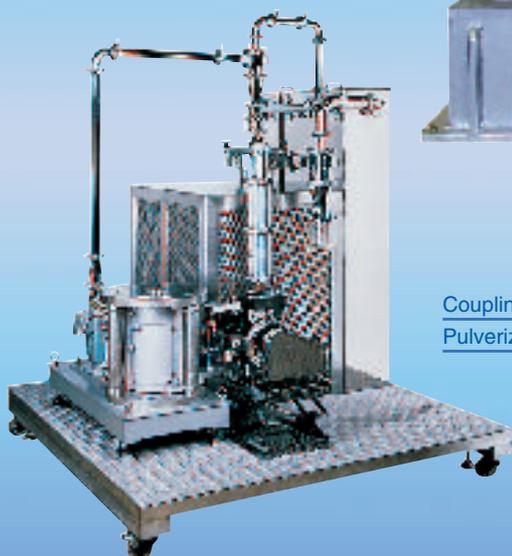
**The Super Rotor - an optimal solution for finely pulverizing materials such as resin. It is a blade mill capable of efficiently pulverizing material which is elastic and/or contains fibers. The powerful spiral flow originated in the narrow clearance between the fixed liner and the rotor with a unique groove shape realizes highly efficient and fine pulverization!!**
