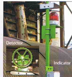
Conveyor Starting Indicator
