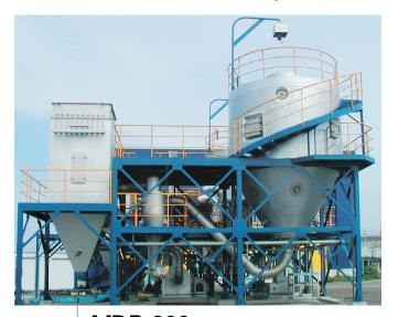
MDP-200 Evaporation capacity : 200kg/hr Drying chamber :  $\phi$ 3.8×5.5m
