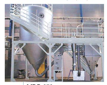
MDP-050 Evaporation capacity: 50kg/hr Drying chamber:  $\phi$ 2.5×4.5m
